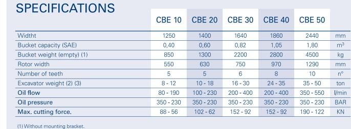
(1) Without mounting bracket.(2) The maximum operating load permitted for the prime mover, when added to the weight of the standard bucket, must match or exceed the weight of the crusher bucket at full load.(3) The user is responsible for checking that the prime mover meets the equipment's specifications and weight requirements.
